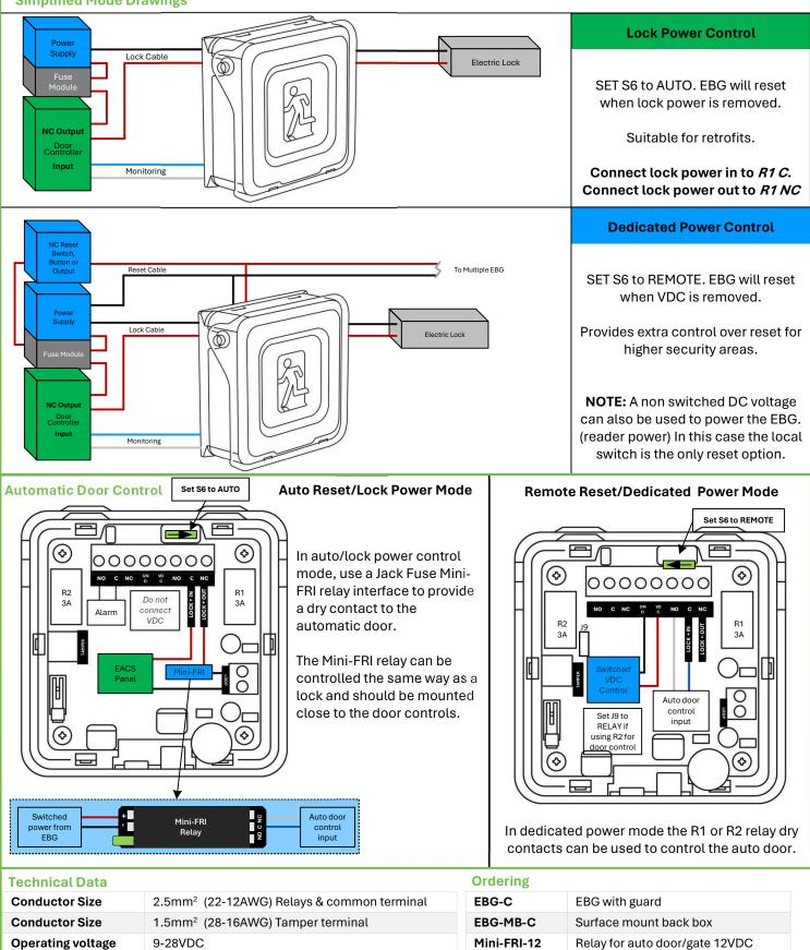
Mini-FRI-24 Dimensions 86X86X40mm (with guard) Relay for auto door/gate 24VDC Sounder Power ~80dB adjustable **Primary materials** Polycarbonate, Polyamide 46, fiberglass Maximum 55mA @ 13.8VDC **Country of origin** China Relay Contacts 3A Max
