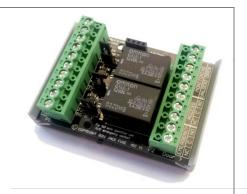
Interface module for connecting automatic doors to access control and fire systems.
