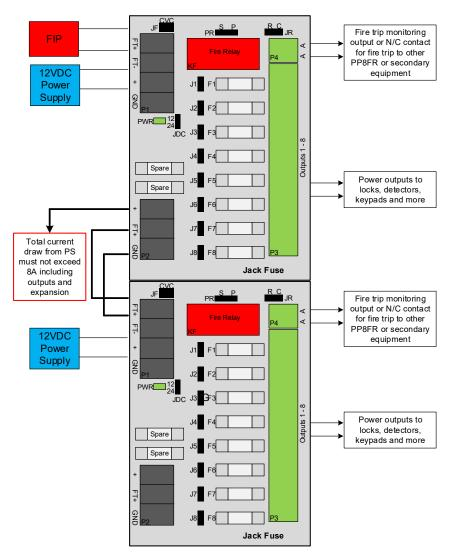
**Additional outputs.** Additional fused power outputs can be added using the expansion boards PP10HD or PP10MG. One or more boards can be added if the total current drawn via the PP8PTC does not exceed the PCB or fire relay limit of 8A. If current draw exceeds limitations an additional PP8FR module can be used.
