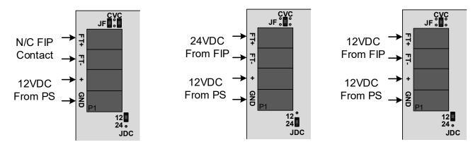
If a normally closed fire trip is used care must be taken to set JDC to the value of the power supply input as this will be used to activate the fire relay.
