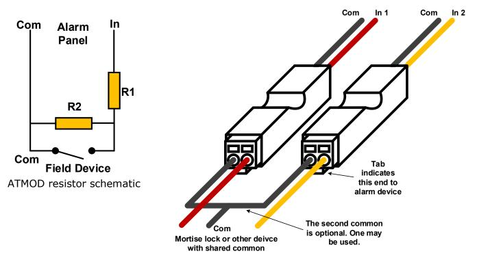
It is a good practice to always wire the common conductor in this method and keep the wire insulation colours the same. *Note: The new ATMOD V4 model features the tab offset to the input or non-common side of the ATMOD.*
