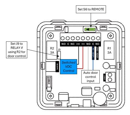
To utilise the dedicated voltage remote reset mode with an automatic door the EBG can provide a dry contact directly from relay 1 or 2.
