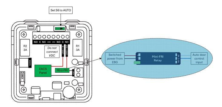
Connect the incoming lock power (from the access control systems) to the EBG J1 terminal ensuring the positive VDC feed from the access control panel is terminated to the common **(C)** terminal of relay 1 marked *LOCK + IN*.
